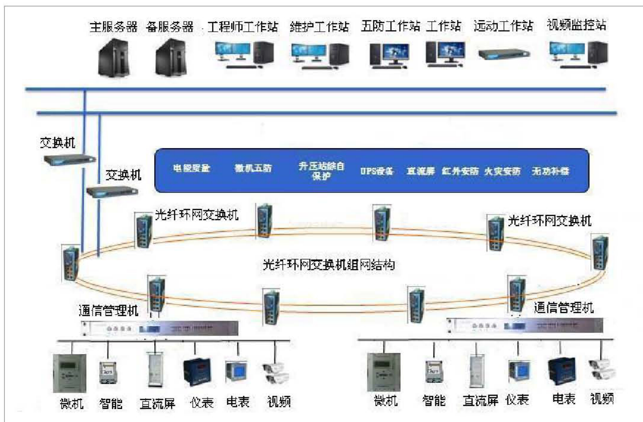
变电站监控系统架构图 Substation Monitoring System Structure
